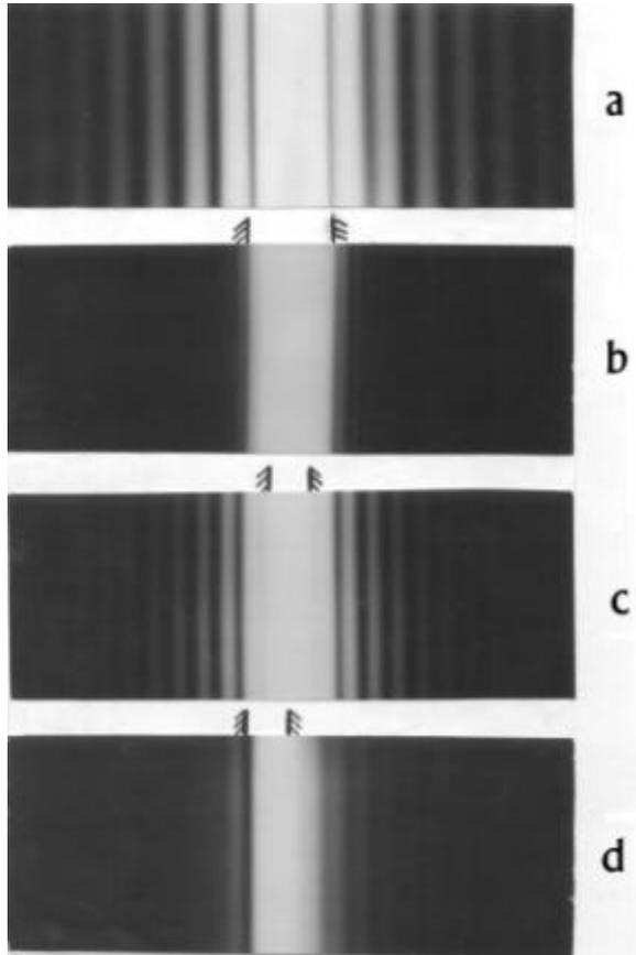
Figure 4. Diffraction-figure at one-coloured inhomogeneous illumination. Experimental arrangement figure 1, but without prism Pr and with green filter. IS = 0.15 mm, b = 100 mm, c = 2 m.
